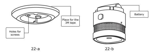
Figure 22 – Fastening of the Smoke Sensor on screws or the 3M tape
