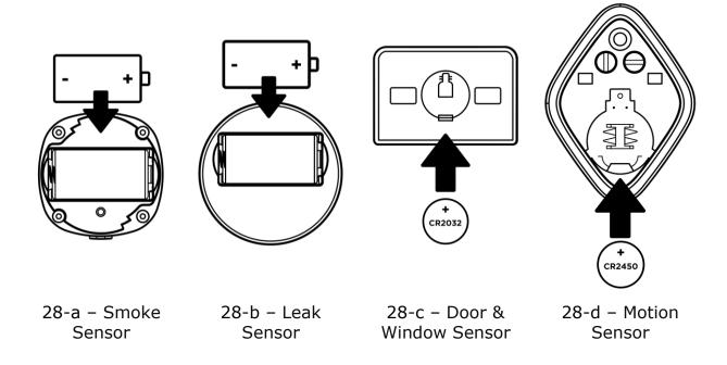
Figure 28 – Positioning of the battery in Sensors
