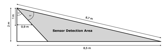
15-c – Details on the vertical detection angle
