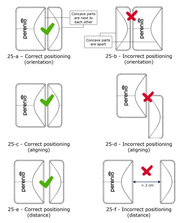
Figure 25 – Installation rules for the Sensor and the Magnet
