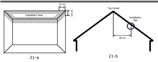
Figure 21 — Installation of the Smoke Sensor on a flat and sloping ceiling
