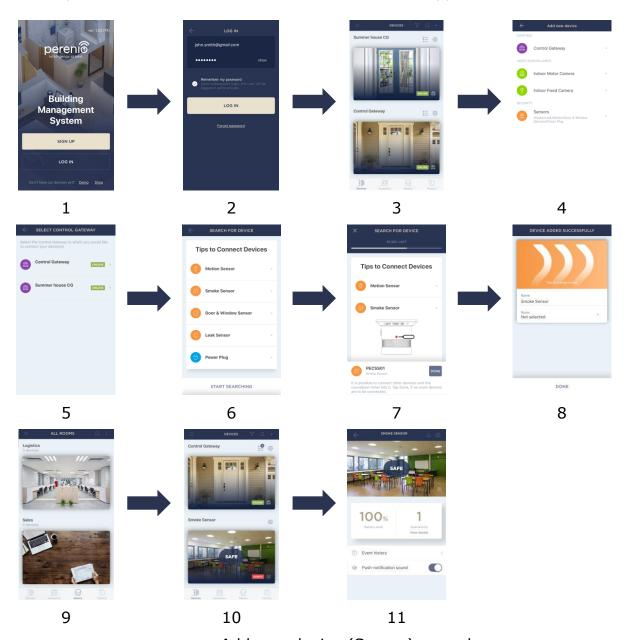
Figure 27 - Add new device (Sensor) procedure
