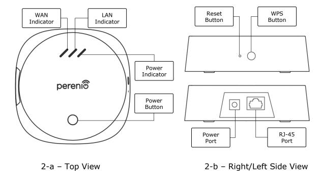
Figure 2 - The PEACG01 Control Gateway Buttons, Ports and Indicators
