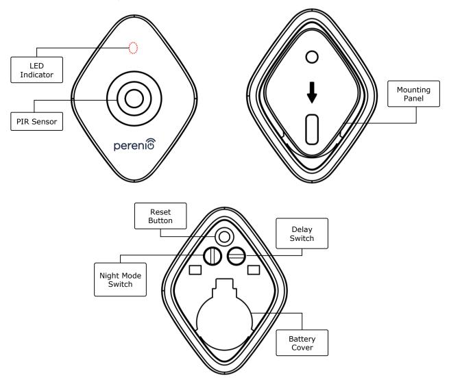
Figure 14 - PECMS01 Motion Sensor Components
