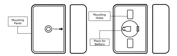
Figure 11 - PECWS01 Door & Window Sensor Components
