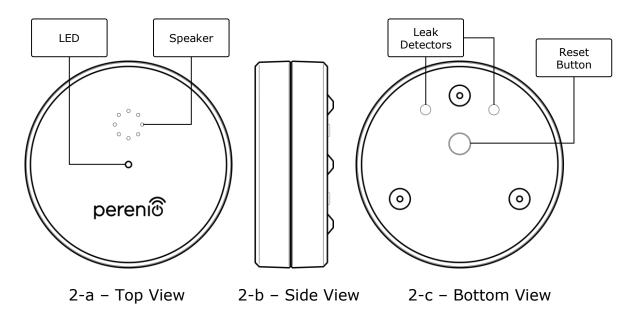
Figure 8 - PECLS01 Leak Sensor Buttons and Indicators
