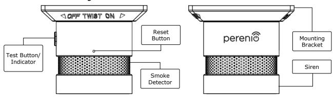
Figure 5 - PECSS01 Smoke Sensor Buttons and Indicators
